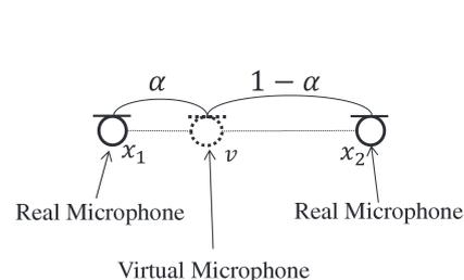
Arrangement of real and virtual microphones [1]
