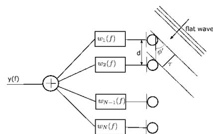
Illustration of the beamforming principle [2]
