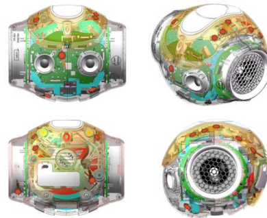
Figure 2: 12-microphone head for the NAO robot.
